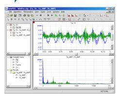
Top graph of a new page shows the selected source signal range, bottom graph shows the calculated results.
